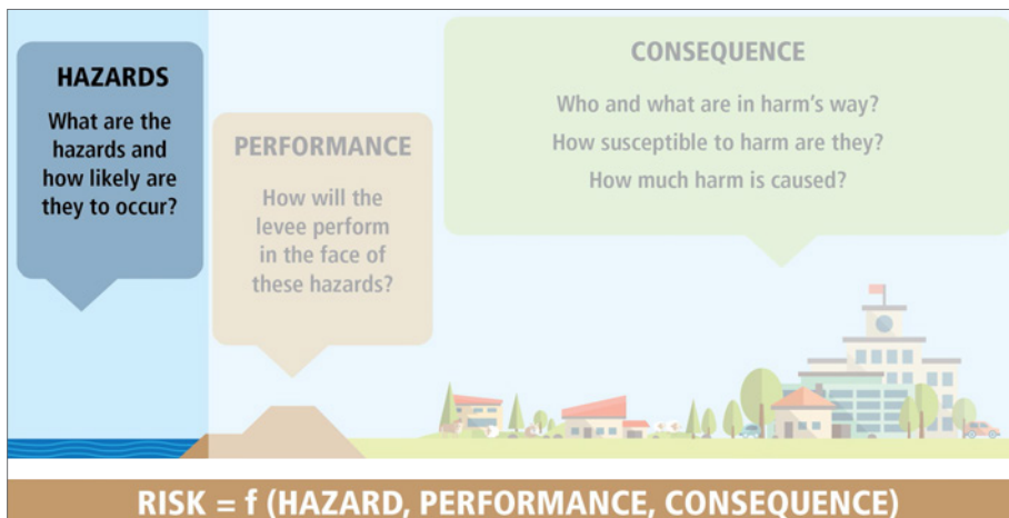
HAZARD COMPONENT OF THE RISK EQUATION USED BY THE USACE LEVEE SAFETY PROGRAM.
