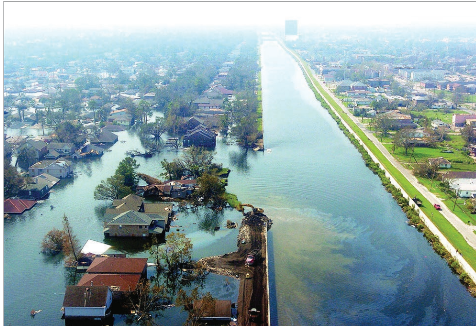
17TH STREET CANAL LEVEE BREACH IN NEW ORLEANS, LOUISIANA, SEPTEMBER 3, 2005 (SOURCE: BRETT DUKE, THE TIMES-PICAYUNE ARCHIVE).
